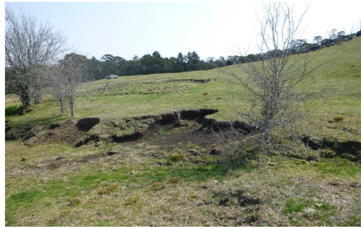
Photo 6: View looking at slumping in a drainage depression in the steep to very steep hillside in the northern part of the site.
